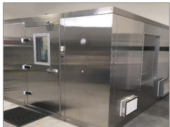
Figure 2: The stainless steel bioaerosol test chamber used for all M50 Testing. Chamber is equipped with HEPA in/out, multiple bioaerosol sampling ports, decontamination and pressure balance. Exterior picture.
