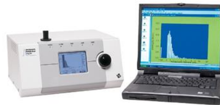
Figure 6. TSI Aerodynamic Particle Sizer (APS) model 3321 used to measure total particle concentration and particle size distribution of the challenge bioaerosol. Range 0.54-20.0 \mu\text{m} aerodynamic diameter, with 1 particle/L detection limits.
